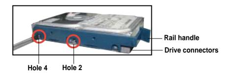
3. Attach **Rail 1** to the side of the drive with two screws as shown. The rail handle should be on the side of the drive connectors.
